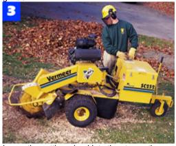
Lower the cutting wheel into the stump, then swing it side to slowly grind the wood into small chips.
